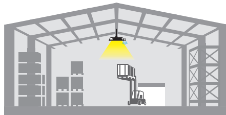
As soon as the sensor detects motion in the scan area, lights will automatically increase to 100%.
